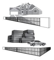
**Class I:** Residential Vehicular Gate Operator – A vehicular gate operator (or system) intended for use in a home of one-to-four single family dwelling, or a garage or parking area associated therewith.
